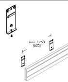
The number of wall fixing brackets depends on the weight load and wall structure. Max. distance 1250 mm. For a heavy weight load, max. distance is 625 mm.
